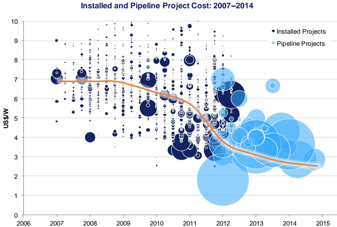
Note: Line illustrates the trend. Representative national average costs for a 20 MW ground-mounted project; EPC includes balance of system and installation costs
